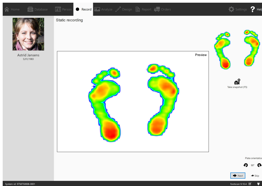
Figure 46: The Static recording takes snapshots of the pressure distribution under the client's feet while standing on the plate.
