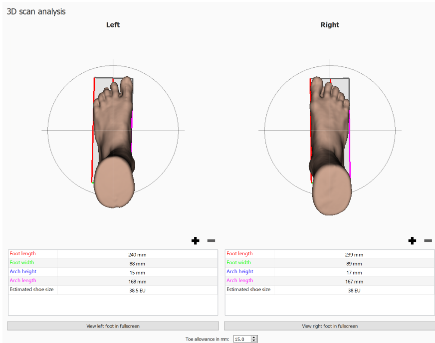
Figure 42: The Both Feet 3D scanner analysis shows the scanned left and/or right foot.
