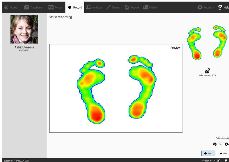
Figure 37: The Static recording takes snapshots of the pressure distribution under the client's feet while standing on the plate.
